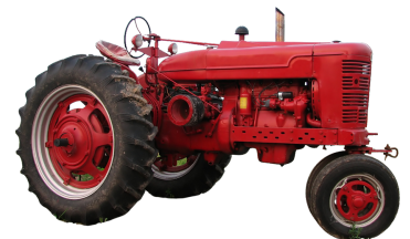
Example of tractor without ROPS
