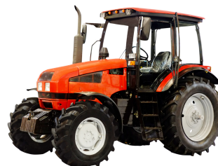
Example of tractor with ROPS
